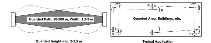
In case of an illegal intrusion, the intruder creates a certain change in the electromagnetic field of the fence. Sensitive circuits detect the change in the electromagnetic field and send out an alarm signal. Since the microwave radiation is invisible, the intruder is unable to sense that the alarm process has been initialized. This feature can be advantageous in certain applications, where recording with a hidden camera is required.
